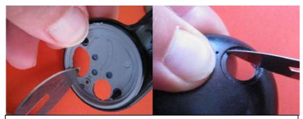
Next smooth edges of the buttons cut out using scalpel or Stanley knife. Gently scrape off rubber remnants from the ledge of the button cut out.
