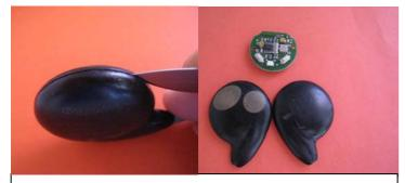
Use scalpel to prise remote open on the split line. You end up with bottom part electronic board and top part with plastic button shell.
