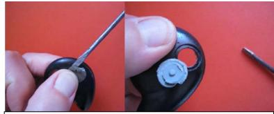
Using a flat screw driver, carefully lift and "shave" off old buttons from plastic casing.
